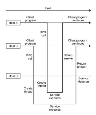
FIGURE 5 MT RPC Server Timing Diagram
