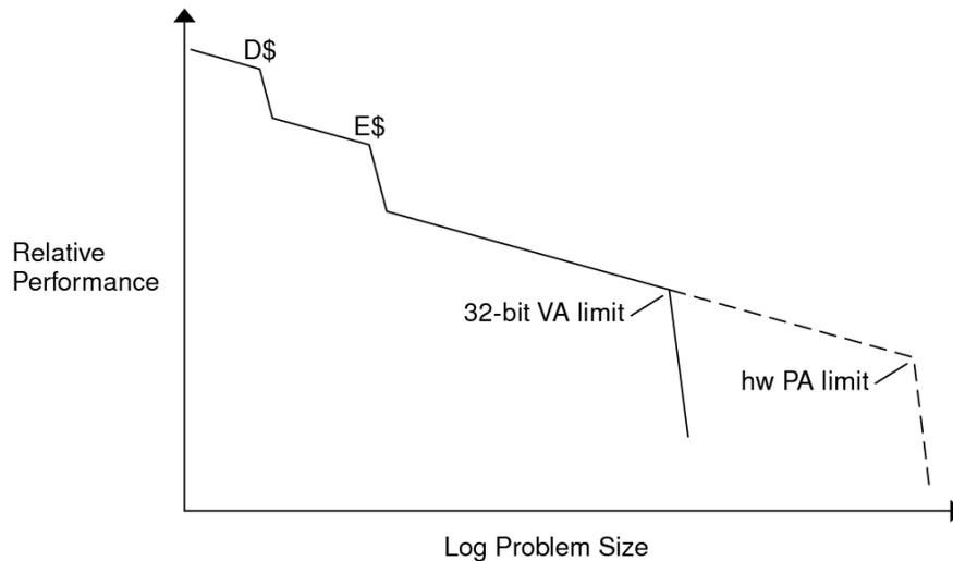
Beyond the 32-bit virtual address limit, applications programmers can still handle large problem sizes. Usually, applications that exceed the 32-bit virtual address limit split the application data set between primary memory and secondary memory, for example, onto a disk. Unfortunately, transferring data to and from a disk drive takes a longer time, in orders of magnitude, than memory-to-memory transfers.
