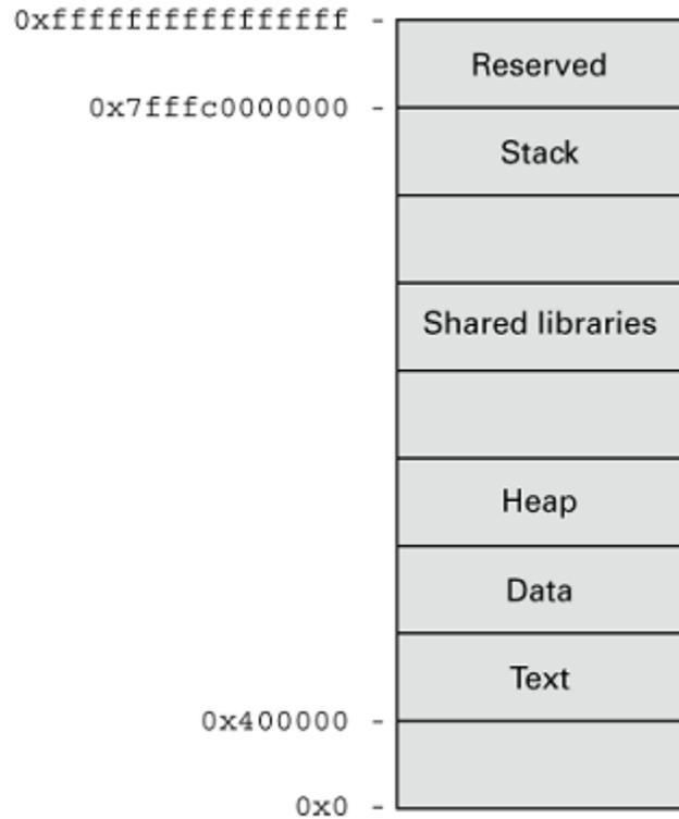
The actual addresses in the figure above describe a particular implementation on a particular machine, and are given for illustrative purposes only.
