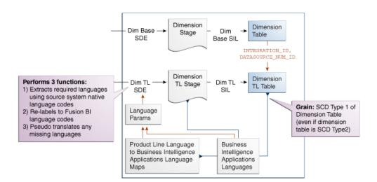
Figure 2–2 Domain ETL Process
