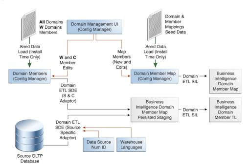
Figure 2–1 Overview of BI Applications Domain ETL Process
