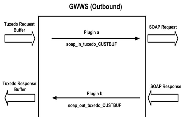
When an Oracle Tuxedo request buffer is delivered to the GWWS server, GWWS tries to find if there is a message conversion plug-in instance associated with the input message conversion of the target service. If there is an associated instance, GWWS invokes the customized (`*soap_out_tuxedo__CUSTBUF`) function implemented in the plug-in instance.
