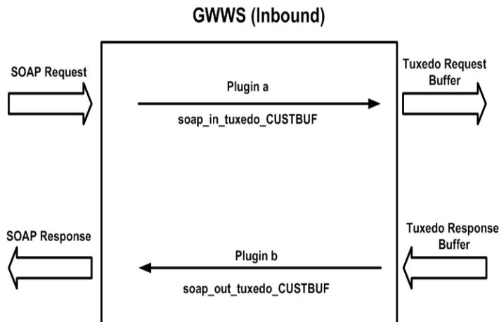
When a SOAP request message is delivered to the GWWS server, GWWS tries to find if there is a message conversion plug-in instance associated with the input message conversion of the target
