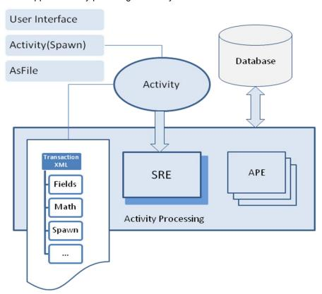
The above diagram illustrates the activity processing at a high level. The transaction XML configures input fields for the activities, the math to transform data, a set of rules to persist the changes, new activities that could be spawned, and so on.
