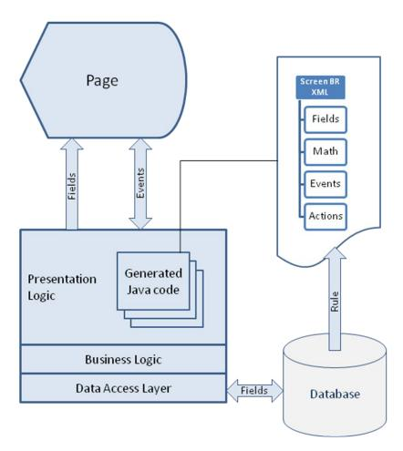
The above diagram illustrates the concept of the page configuration. A screen business rule is used to create a set of fields that are displayed on a page. A set of Java classes, generated at run-time and based on the rule's logic, is responsible for handling screen events – page load, page submit and field value changes.
