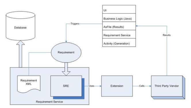
The Requirement Service is the heart of requirement processing. The service is a state machine executor that moves requirements from one state to another according to the requirement XML. The Requirement Service is built around the Shared Rules Engine. OIPA extensions are used to call out to external services and perform what is needed to obtain requirement results. Requirements can be created, or their processing resumed, by
