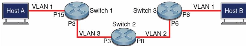
In this topology, P15, P3, P6, and P8 represent ports on the SEFOS switches. Switch 1 and switch 2 are NEM switches, and switch 3 is a TOR switch.
