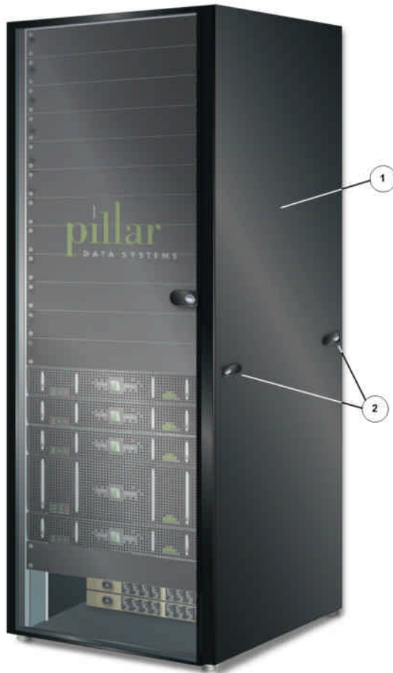
Figure 4 Sample 42U side panels
