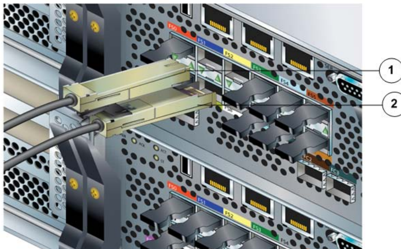
Figure 55 SFP module insertion
