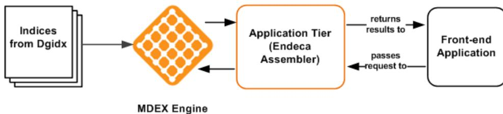
The MDEX Engine is designed to be stateless. This design requires that a complete query be sent to the MDEX Engine for each request. The stateless design of the MDEX Engine facilitates the addition of MDEX Engine servers for load balancing and redundancy. Because the MDEX Engine is stateless, any replica of an MDEX Engine on one server can reply to queries independently of a replica on other MDEX Engine servers.
