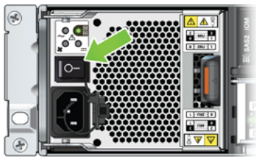
Figure 5.4 Sun ZFS Storage Appliance Circuit Breakers
