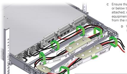
B Open the CMA cable covers, route server cables through the CMA's cable troughs, close the cable covers, and secure the cables with the six Velcro straps. Start with the frontmost cable trough, then through the small cable trough, and finally through the rear-most cable trough.
