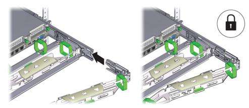
F Remove the tape that secures the slide-rail latching bracket to connector D and ensure that the latching bracket is properly aligned with connector D.
