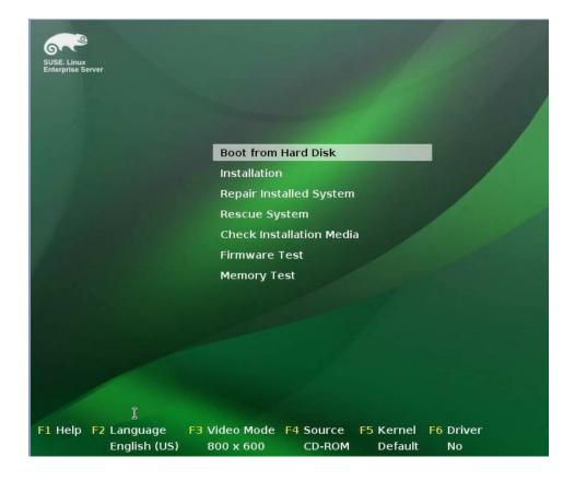
5. In the boot screen, use the tab key to select the second option Installation, then press Enter.
