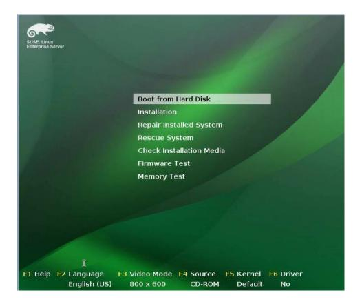
5. In the boot screen, use the tab key to select the second option Installation, then press Enter.
