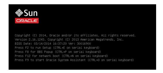
2. When prompted in the BIOS screen, press the F2 key to access the BIOS Setup Utility.
