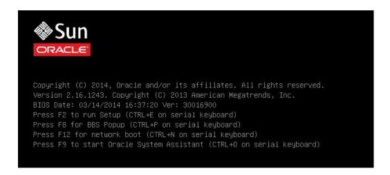
25. To access the BIOS Setup Utility so that you can set the server to boot from the operating system you just installed, press the F2 key.
