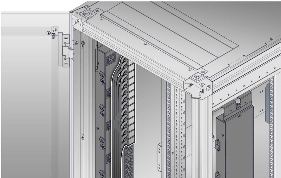
**2. Install the slide-rails into the rack.**
