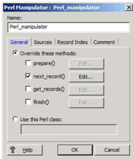
Clicking **Edit** for the `next_record()` method displays the **Method Override editor**, which contains the Perl code shown below. This code removes records with the property named Delete This Record.
