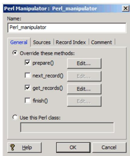
Clicking **Edit** for the `prepare()` method displays the **Method Override** editor which contains the Perl code shown below. This code sets a flag for later manipulation on the first call of `get_records()`.
