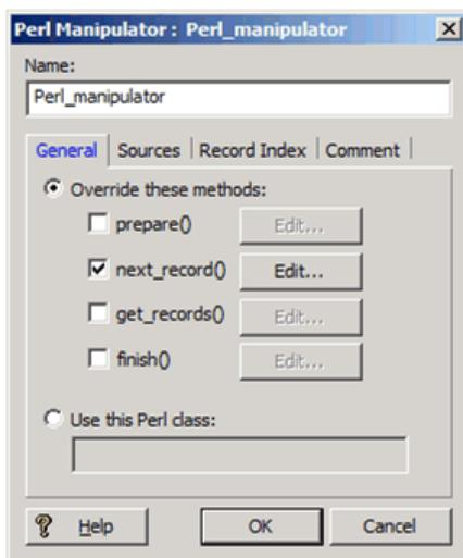
Clicking **Edit** for the `next_record()` method displays the Method Override editor which contains the Perl code shown below. This code removes the Password property from each record.
