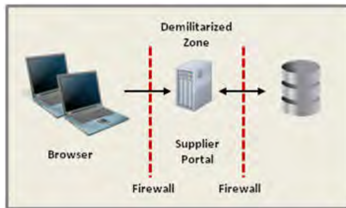
Figure 2-3 Deploying Supplier Portal in DMZ
