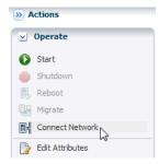
**4.** Only available networks that are not currently connected to the selected logical domain appear in a table. Select the networks to which you want to connect the guest, and click Connect To Network to finish.
