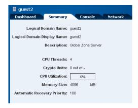
When an Oracle VM Server for SPARC in the server pool fails, the logical domains that have been enabled for automatic recovery are recovered and started on another Oracle VM Server in the server pool without any user intervention.
