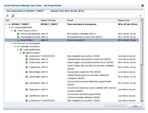
From the job details, you can view that the server *smt4-15* is powered off according to the server pool policy. The logical domain *guest2* recovery is initiated and created successfully on the Control Domain *smt4-14* in the server pool. When the logical domain *guest2* is recovered, the server pool status is as in the following figure:
