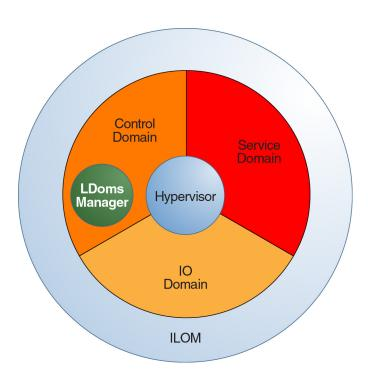
**FIGURE 1-3** Components of the Execution Environment
