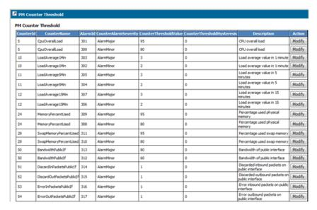
Figure 2: Counter Threshold Window from the WebCI
