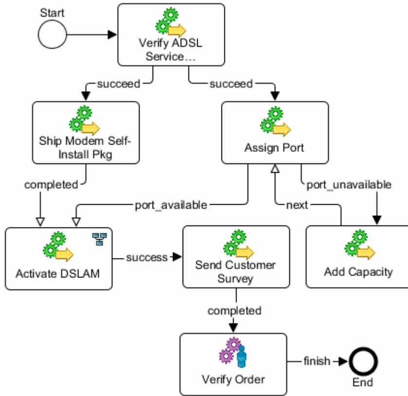
This process manages the fulfillment of a request for an ADSL service:
