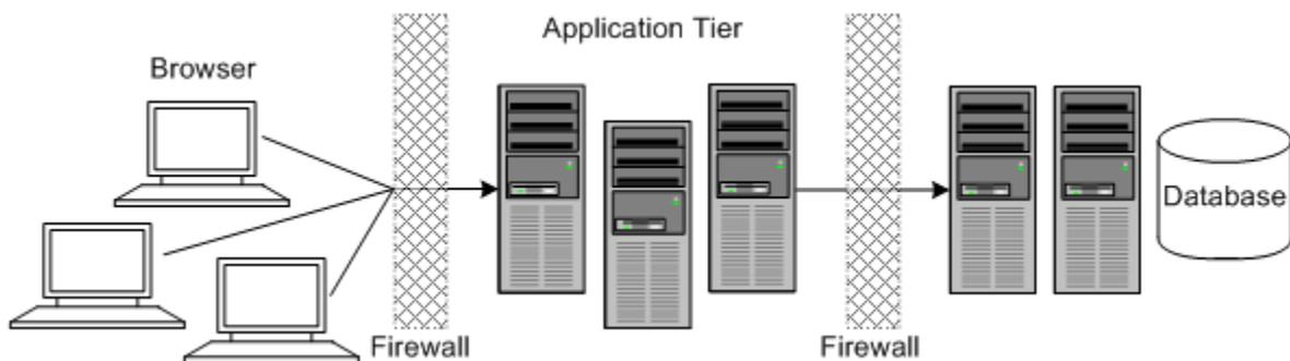
In this topology, the application tier is isolated by firewalls from both the Internet and the intranet. The database and servers are protected from potential attacks by two layers of firewall. Both firewalls can be configured to block known illegal traffic types. The two layers of firewall also provide intrusion containment. Although there are more components to secure, and more ports must be opened to allow secure communication between the tiers, the attack surface is spread out.
