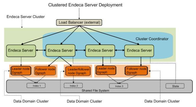
In this diagram, starting from the top, the following components of the Endeca Server cluster deployment are included:
