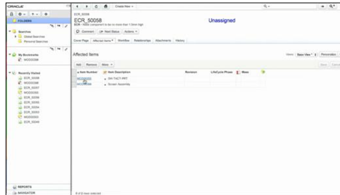
Figure 9 After creation from AutoVue, both the selected Part and Assembly Part are added to Affected Items
