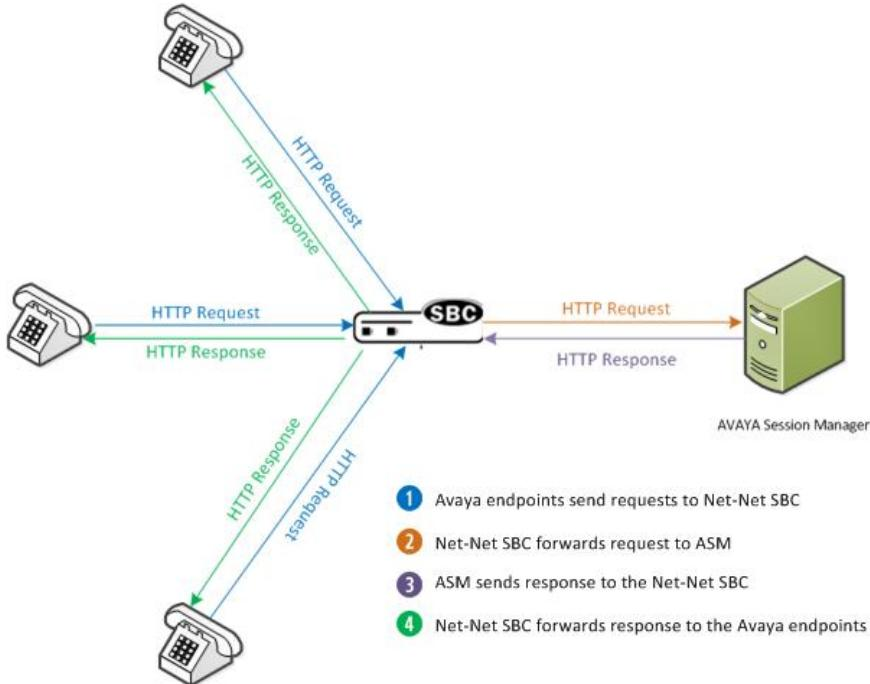
The following is the call flow that occurs as the HTTP/HTTPS requests and responses are passed between the Avaya endpoints, the Oracle SBC, and the ASM.
