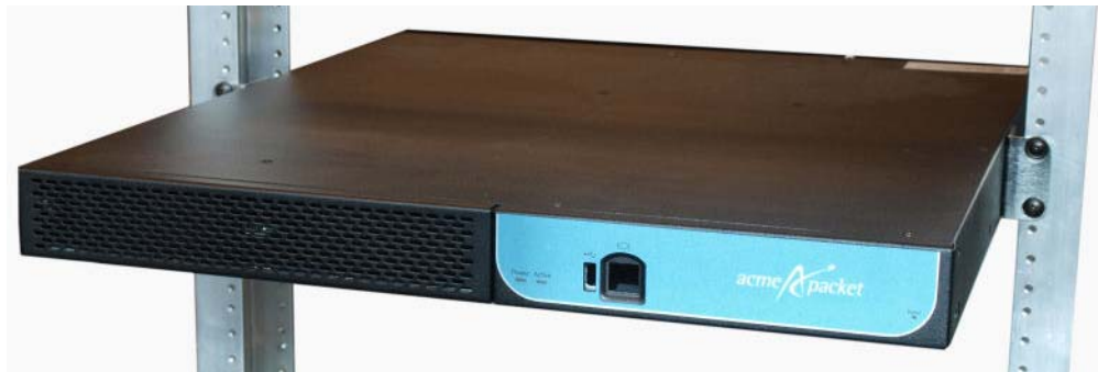
Figure 2 - 58. Acme Packet 3820 Center-Mounted in a Two-Post Equipment Rack
