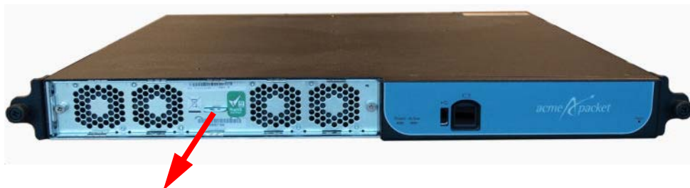
Figure 4 - 103. Removing the Fan Assembly
