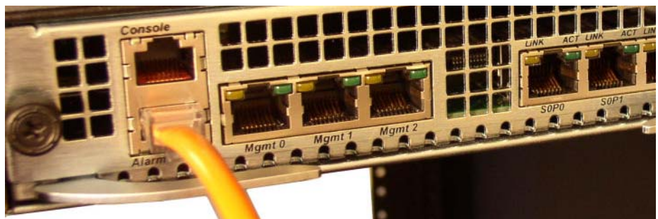
Figure 2 - 78. Connected Alarm Cable
