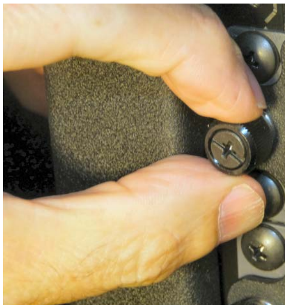
Figure 1 - 13. Securing the Chassis to the Rack
