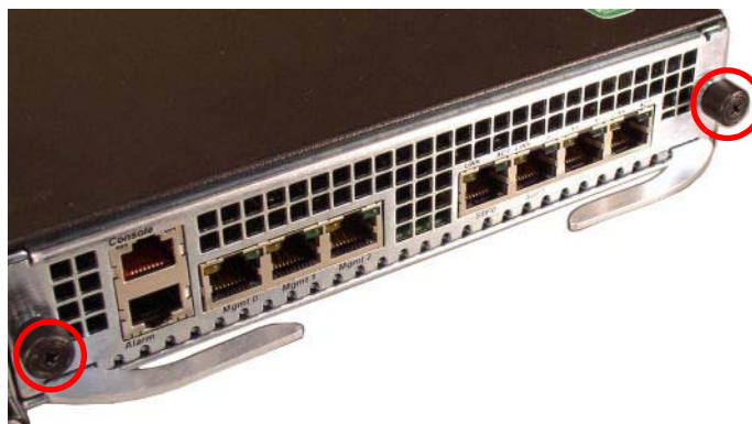
Figure 4 - 119. Securing the NIU
