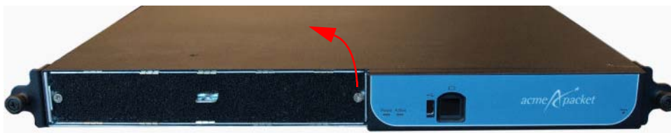
Figure 4 - 101. Removing the Air Filter
