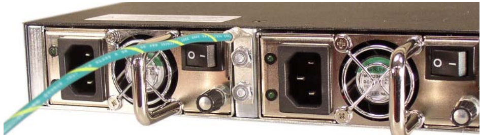
Figure 2 - 61. Ground Cable Secured on Ground Posts
