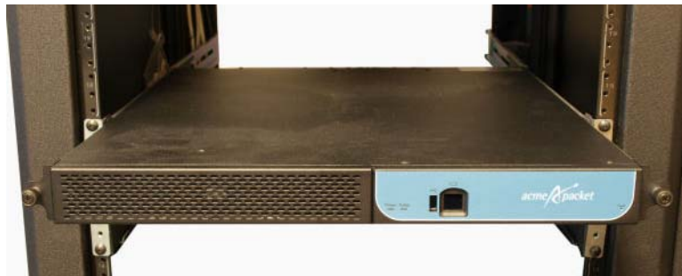
Figure 2 - 54. Installing the Acme Packet 3820 into the Equipment Rack
