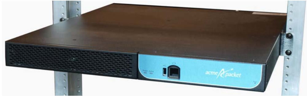
Figure 2 - 55. Center-Mounted Acme Packet 3820
