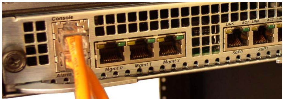
Figure 2 - 75. Console Cable Installed
