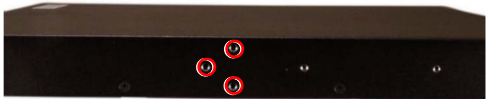
Figure 2 - 56. Tapped Holes in Acme Packet 3820 for Center Mounting the Chassis
