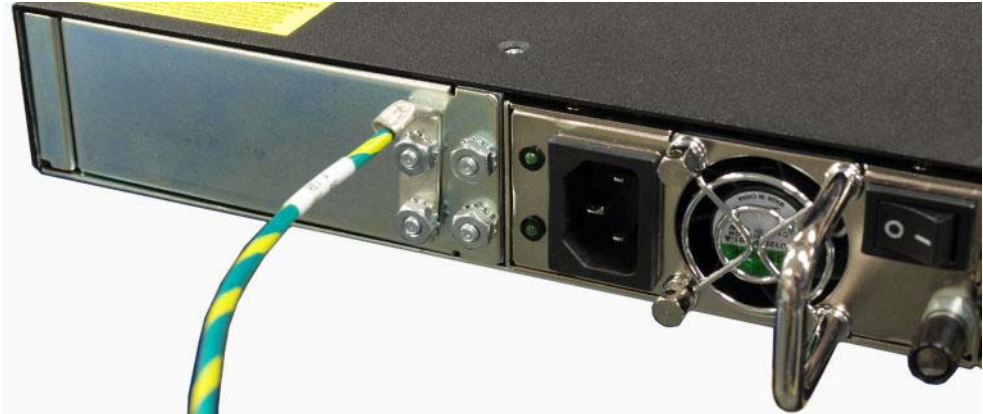
Figure 2 - 64. Ground Cable Secured to the Ground Posts
