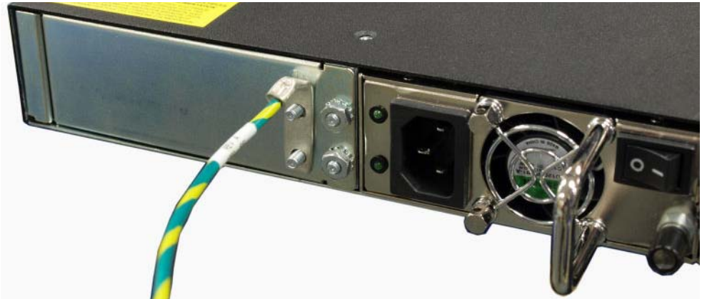
Figure 2 - 63. Aligning the Ground Cable to the Ground Posts
