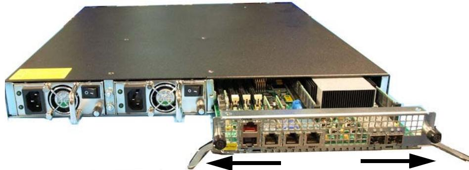
6. The NIU card is removed from the chassis and moved to an ESD safe location.
