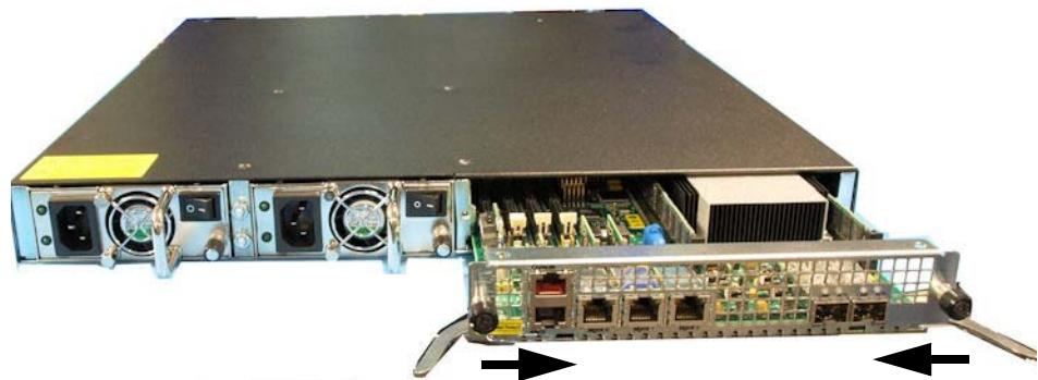
5. With a #2 phillips head screw driver, screw in the two screws so the 10-gigabit NIU card is secured in the chassis.
