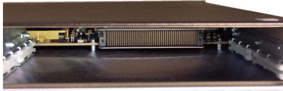
2. Insert the 10-gigabit NIU card into the chassis with both sides of the 10-gigabit NIU card inserted into the guide rails.
