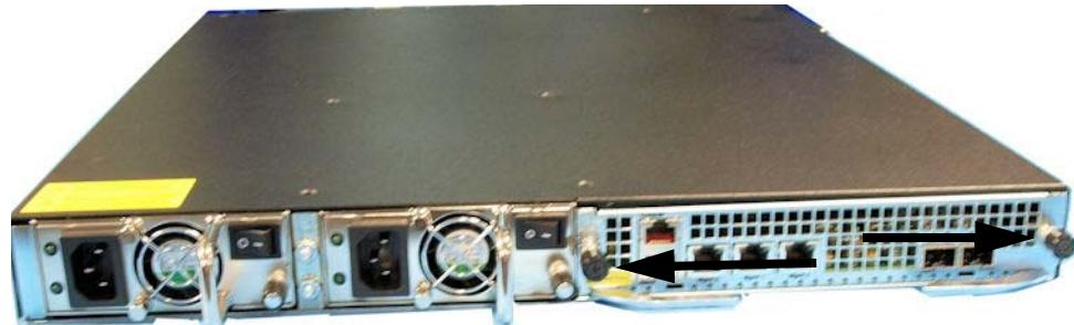
4. Pull the two ejector handles out and away from the chassis at the same time to disengage the 10-gigabit NIU card from the midplane and chassis.
