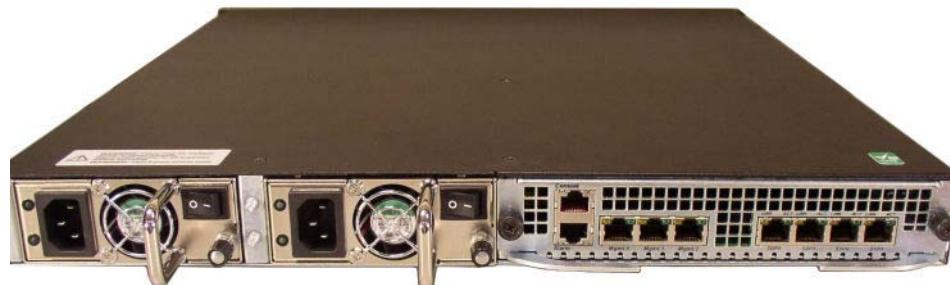
3. Unscrew the two thumb screws located on each side of the ETC NIU with a #2 Phillips head screwdriver. The screws are spring-loaded and will be pushed forward, but will not fall out of the ETC NIU.
