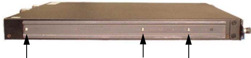
2. Remove the left rack ear by unscrewing the three screws.
