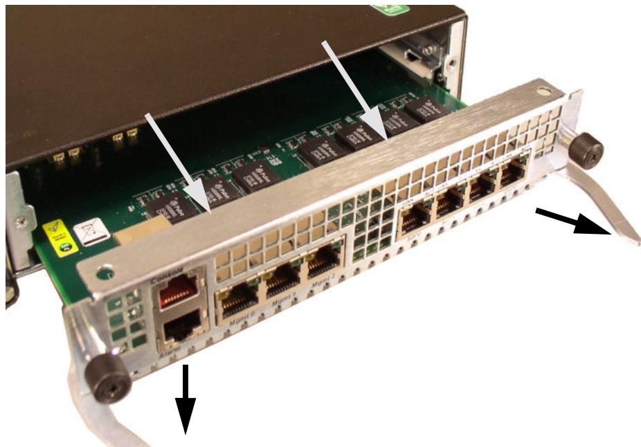
6. The Transcoding NIU card is removed from the chassis and moved to an ESD safe location.
