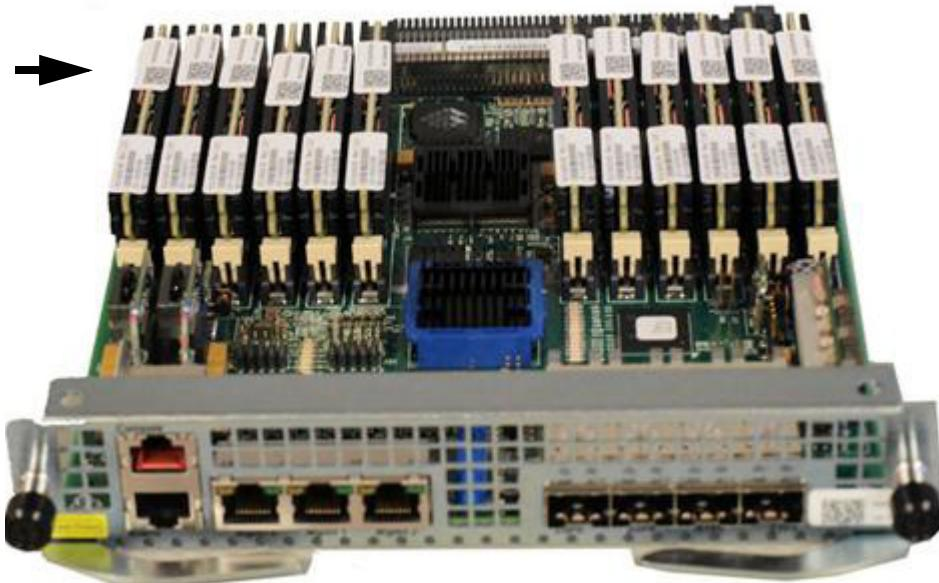
Transcoding NIU with no DSP modules installed in slots **0-11**. The arrow is indicating the location of slot 0.
