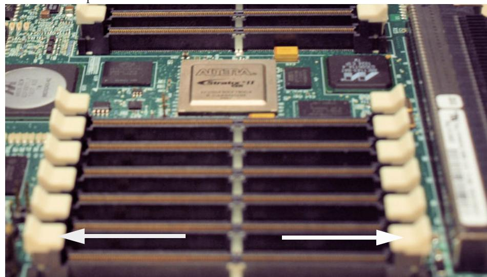
4. The two white ejector handles are in the extended position and ready for the DSP module to be inserted into the socket.
