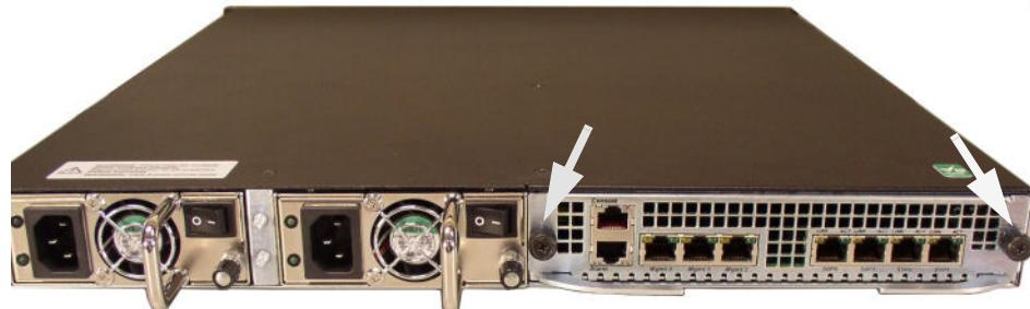
4. Pull the two ejector handles out and away from the chassis at the same time to disengage the Transcoding NIU card from the midplane and chassis.
