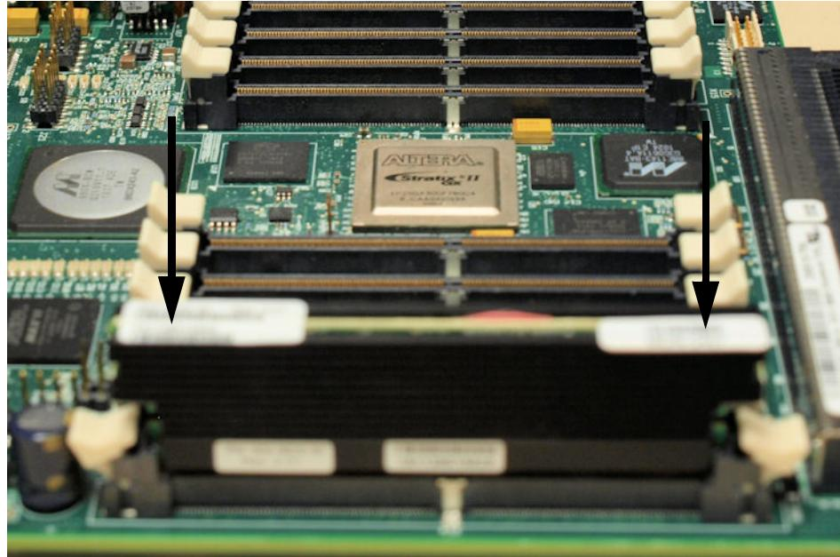
8. As you press down evenly across the top of the DSP module, the two white ejector handles will move up and lock the DSP module into the socket.
