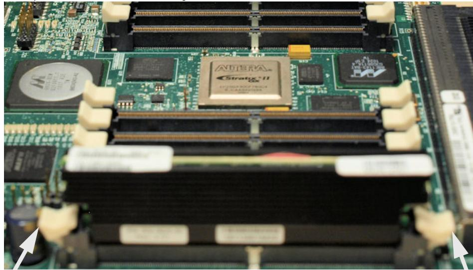
9. The two white ejector handles and the DSP are locked into the correct position in the socket. Repeat these steps for as many DSP modules you have, populating in slot 0 through 11 or less.
