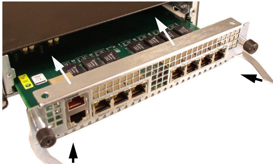
5. With a #2 phillips head screw driver, screw in the two screws so the Transcoding NIU card is secured in the chassis.
