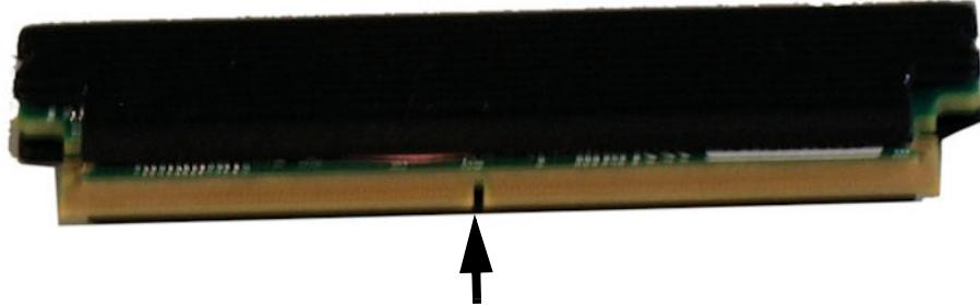
6. Make sure the keyed position is correct on the DSP module and the socket, then insert the DSP module into the socket.
