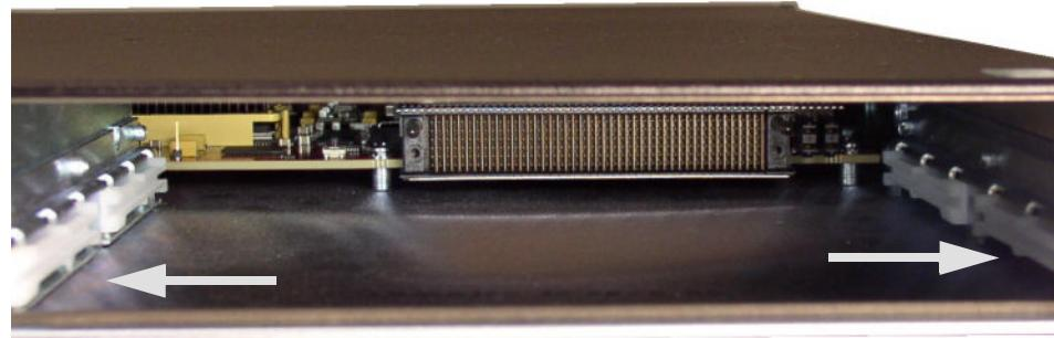
2. Insert the Transcoding NIU card into the chassis with both sides of the Transcoding NIU card inserted into the guide rails.
