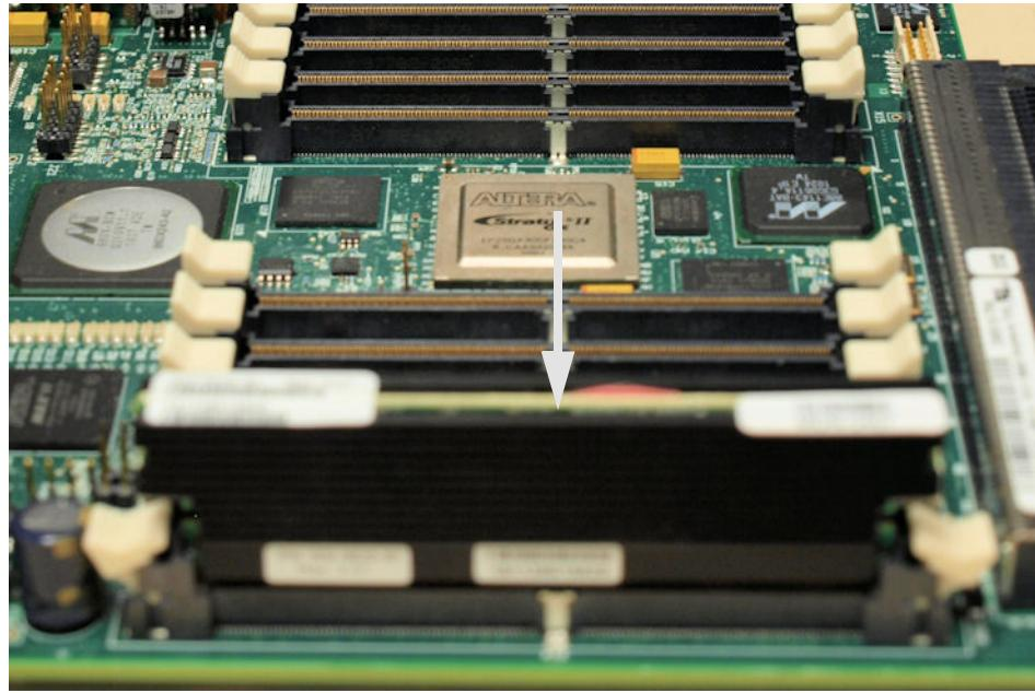
7. Once the DSP module is inserted into the socket properly. Apply pressure evenly across the top of the DSP module until it is inserted into the socket.
