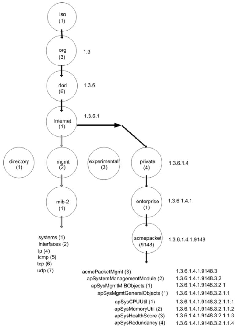
The diagram shows the Acme Packet node has the value 9148. This node is the highest level of the private (proprietary) branch containing Acme Packet managed objects. The number 9148 was assigned to signify Acme Packet's private branch by the Internet Assigned Numbers Authority (IANA).
