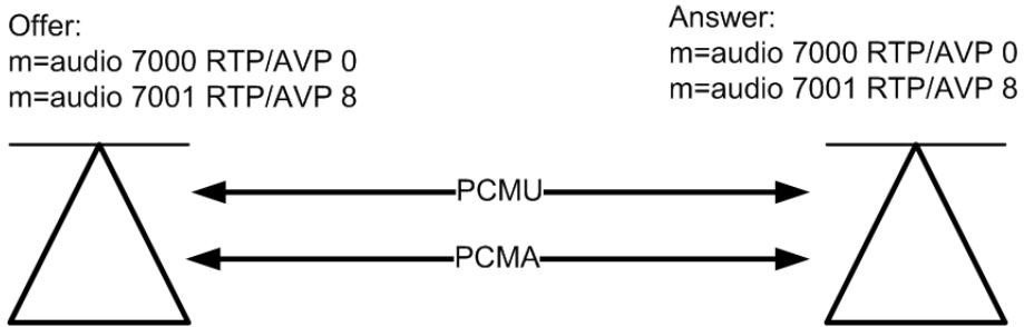
If the session originator and terminator in the previous diagram exist in two different realms, you must execute the **show sip codecs** command twice, once for each realm. A single PCMU count and a single PCMA count will be reflected in each respective query because two m= lines emanate from each realm.
