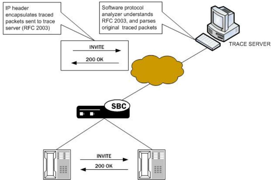
It is possible that—for large frames—when the Net-Net SBC performs the steps to comply with RFC 2003 by adding the requisite header, the resulting packet might exceed Ethernet maximum transmission unit (MTU). This could result in packets being dropped by external network devices, but widespread support for jumbo frames should mitigate this possibility.
