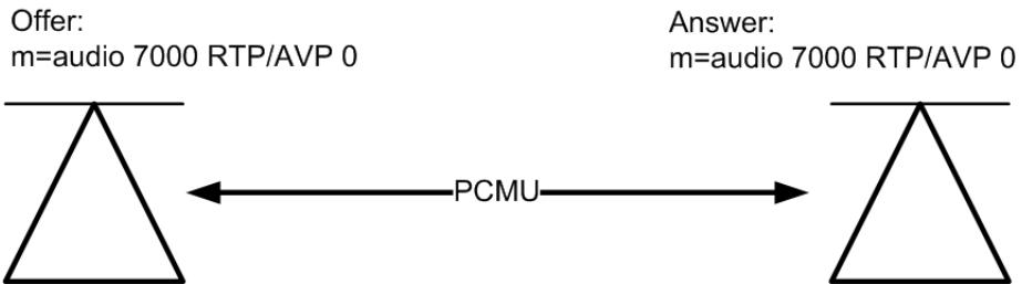
If the session originator and terminator in the previous diagram exist in two different realms, you must execute the **show sip codecs** command twice, once for each realm. A single PCMU count will be reflected in each respective query because only one m= line emanates from each realm.
