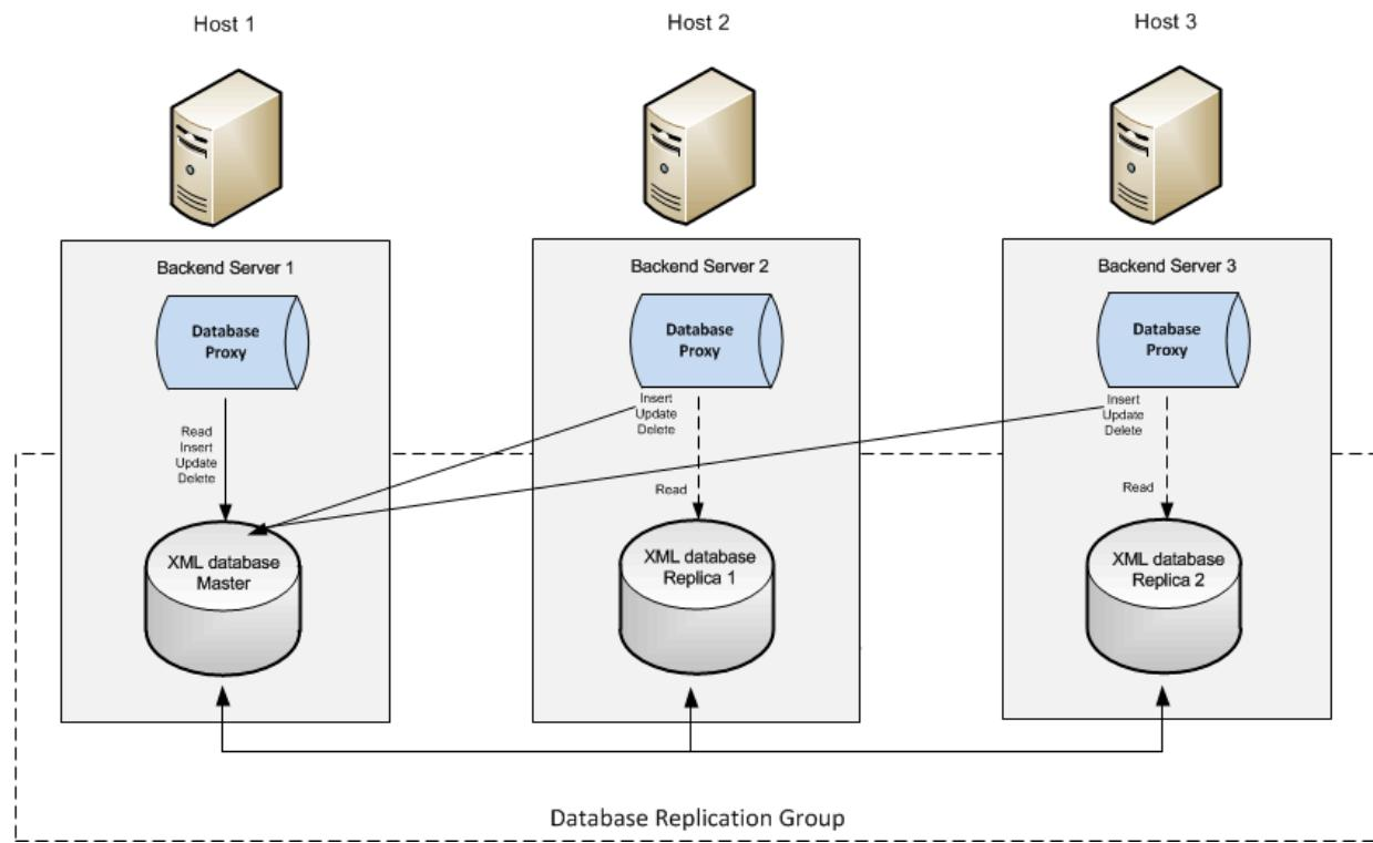
As illustrated in the diagram above, the cluster consists of three host systems. The database replication mechanism shown demonstrates the following points:
