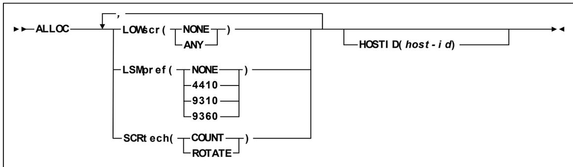
FIGURE 7-1 ALLOC syntax
