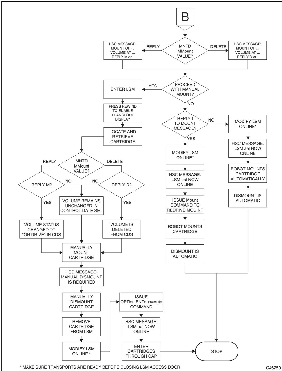
FIGURE 8-3 Manual Mode Flow Chart - Manual Mount/Dismount
