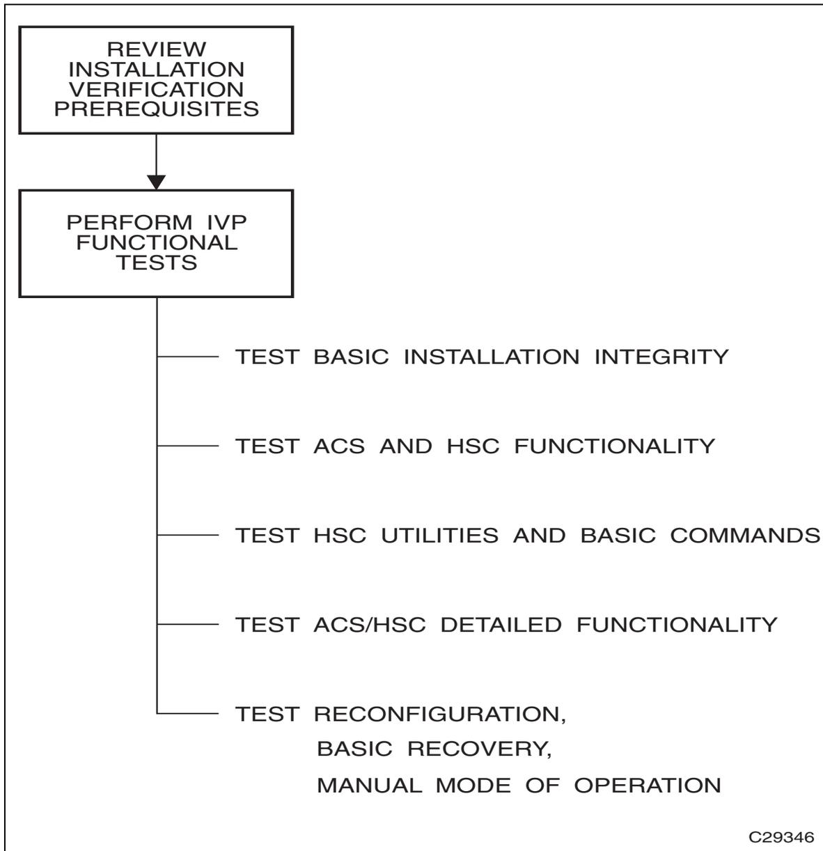
FIGURE 11-1 Installation Verification Flow Diagram
