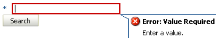
Figure 4–10 Client-Side Validation Displays an Error Without a Trip to the Server
