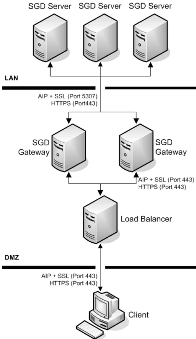
Configuring a load-balanced deployment involves configuring the connections shown in [Table 2.2, "Connections For a Load-Balanced Deployment of the SGD Gateway"](#).
