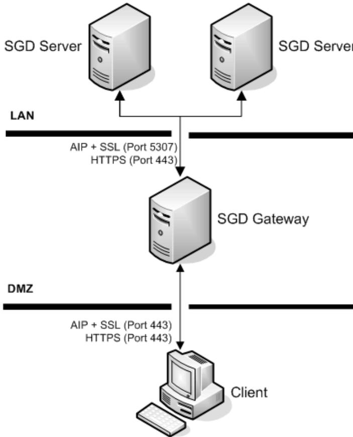
Configuring a basic deployment involves configuring the connections shown in [Table 2.1, “Connections For a Basic Deployment of the SGD Gateway”](#).
