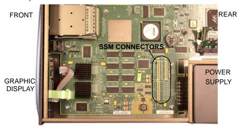
2. Note the three board-to-board connectors in the following photograph. This photograph shows the bottom of the SSM. When attaching the SSM to the motherboard, these board-to-board connectors set closer to the Net-Net 4250 SD's power supply, NOT the graphic display.
