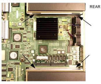
3. Secure the lid in place by repeating the opposite motion used for removing it. Push the lid downward and toward the front of the chassis in one sweeping motion.
