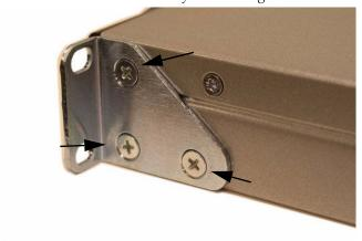
2. Remove the right rack ear by unscrewing the three screws.
