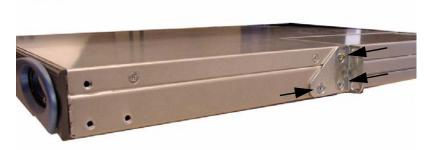
2. Remove the right rack ear by unscrewing the three screws.
