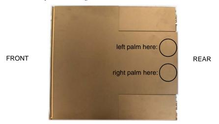
4. Force a down and rearward pressure to move the chassis lid backward by about 1/4". The lid will make a snapping sound after it travels fully toward the chassis rear. This requires moderate force.
