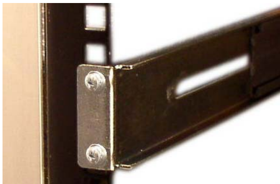
Figure 4 - 56. Installed Slide Rail in a Square-Hole Rack - Rear Mount Point
