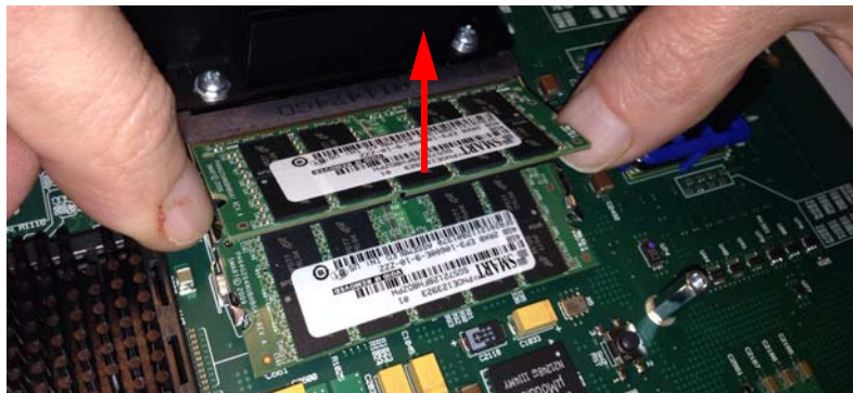
Figure 6 - 113. Releasing Spring-Loaded SODIMM Clips
