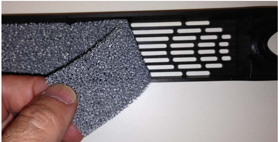
Figure 6 - 143. Removing the Air Filter from Behind the Front Bezel
