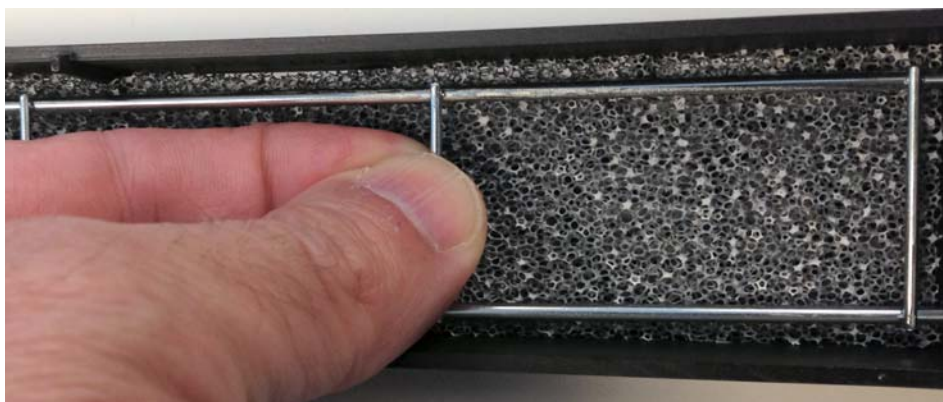
Figure 6 - 142. Removing the Air Filter Wire Retainer from Behind the Front Bezel
