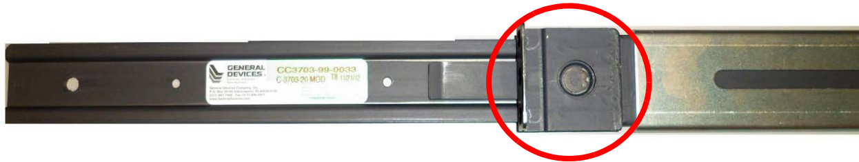
Figure 6 - 90. Locking Clip Fastens the Chassis and Rack Slide Rails
