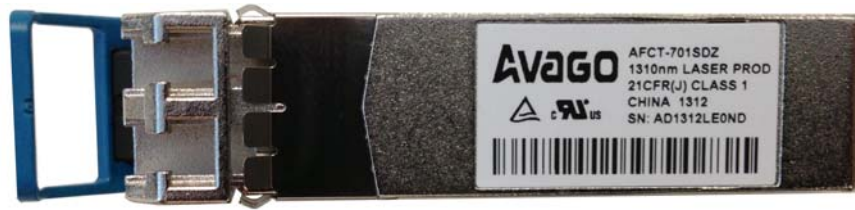
Figure 6 - 124. 10 Gigabit Single Mode SFP+ Transceiver (Blue Bale Clasp Latch)
