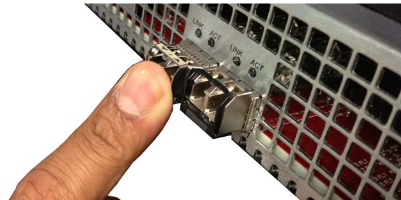
Figure 6 - 131. Seating the SFP+ Optical Transceiver
