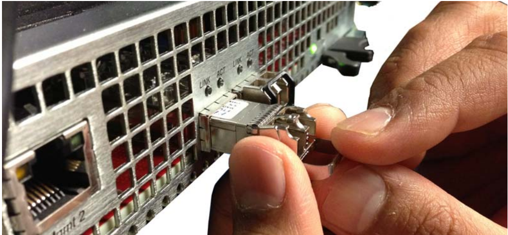
Figure 6 - 129. Removing the Optical Transceiver
