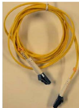
Figure 6 - 126. 10 Gb Yellow Fiber Optic Cable for Use with LX Transceivers
