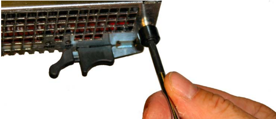
Figure 6 - 104. Tightening NIU Thumbscrews
