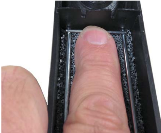
Figure 6 - 145. Replacing the Air Filter Bracket Behind the Air Filter
