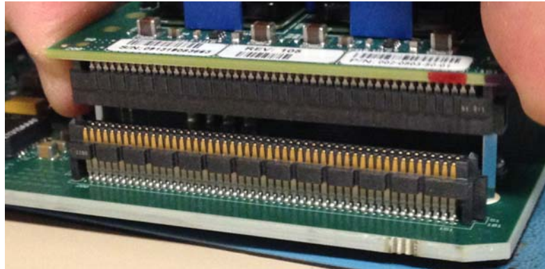
Figure 6 - 107. Installing the SSM3 Module
