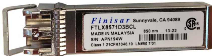
Figure 6 - 123. 10 Gigabit Multi Mode SFP+ Transceiver (Black Bale Clasp Latch)
