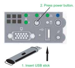
Warning: **DO NOT** remove the USB stick until the system has completed the bootup sequence, which may take up to ten minutes.
