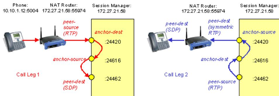
If the OS-E determines that the RTP comes from a different IP address than was signaled in SIP, then it knows that the endpoint is behind a NAT device. In this case it will send the return path media back to the same IP address and port as the outbound path, using symmetric RTP, provided that symmetric RTP has been enabled for media in the session configuration. In these cases the use of RTP is shown as follows:
