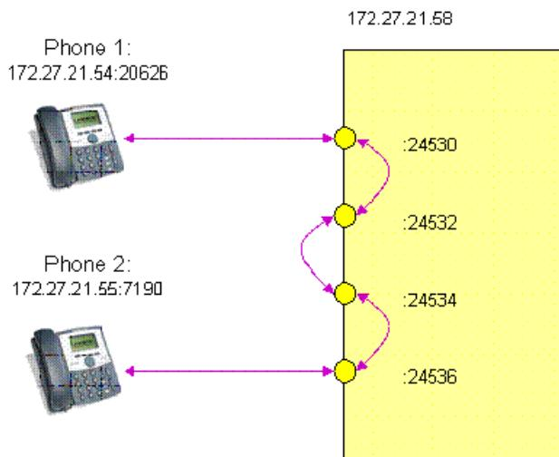
If the OS-E determines that the two halves of the same call originate behind the same NAT device (because the public IP addresses of the called and calling parties are the same), it will direct the two endpoints to send media to each other directly using their private IP addresses, and will not anchor the media, provided that media anchoring has been set to *auto-anchor* in the session configuration.
