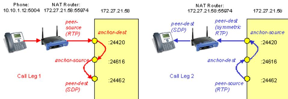
If the OS-E determines that two separate calls are the two halves of the same call (which is the case when the calling and called party are connected to the same OS-E system), it will link the media ports for the two calls as shown below in the image below.
