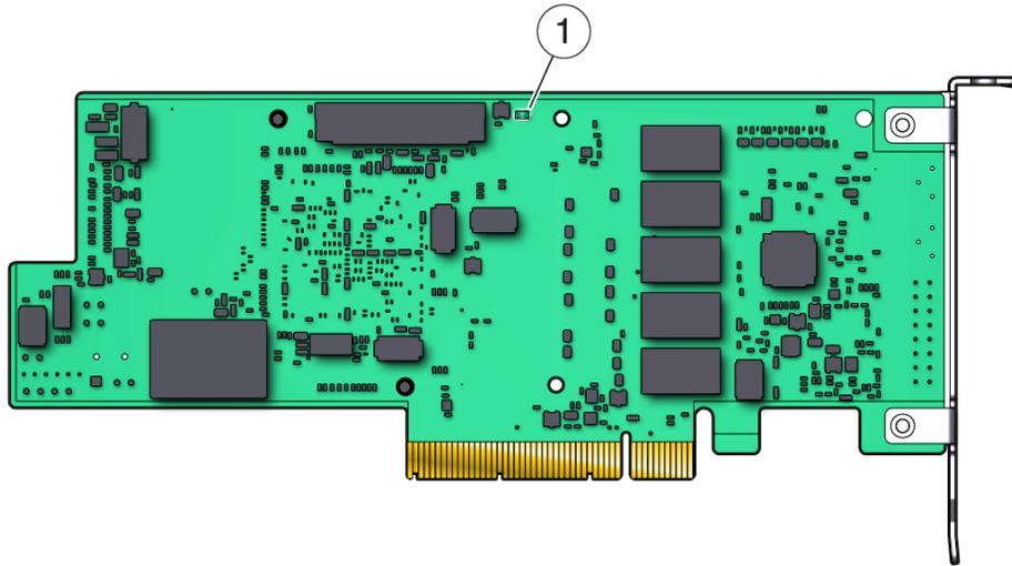
A green System Heartbeat LED (CRT4B1) indicates that the SAS3108 RAID-on-chip (ROC) ASIC is operating normally.
