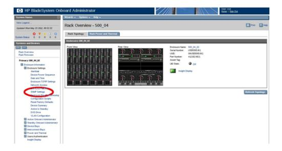
All configured SNMP trap destinations will be shown in the box in the center of the SNMP Settings page.
