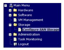
From the **Storage** Configuration drop down menu choose SAN configuration file and press Configure Storage.
