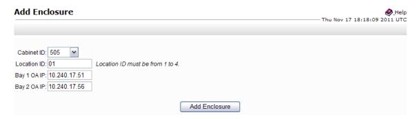
**Note:** Location ID is used to uniquely identify an enclosure within a cabinet. It can have a value of 1, 2, 3, or 4. The cabinet ID and location ID will be combined to create a globally unique ID for the enclosure (for example, an enclosure in cabinet 502 at location 1, will have an enclosure ID of 50201).
