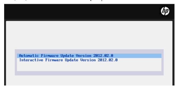
If no key is pressed in 30 seconds the system will automatically perform an Automatic Firmware Update.
