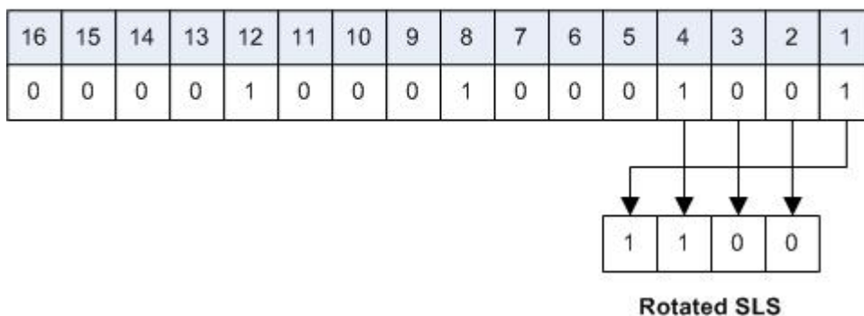
Figure 22: Example of Bit Rotation
