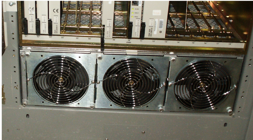
Figure 64: Fan tray inserted into fan tray bracket in the frame - front view
