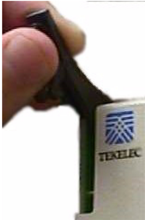
Figure 28: Push Inject/Eject Clamps Outward
