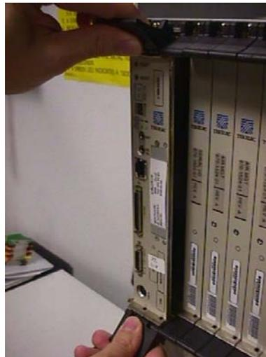
Push the card along the length of the card guides until the rear connector on the card begins engaging the mating connector on the backplane.
