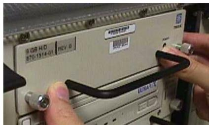
Press the faceplate near the areas where the handle is in contact with the faceplate.
