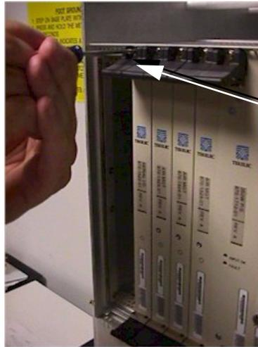
Loosen the captive screws until they no longer engage the threads.
