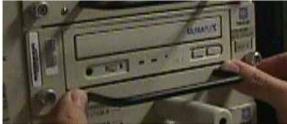
Press the faceplate near the areas where the handle is in contact with the faceplate.
