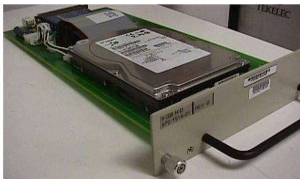
15. Use one hand to support the card assembly from underneath and the other hand to grasp the faceplate handle (see Figure 6-42).
