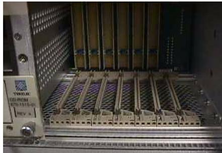
← Prior to inserting the replacement card, check connectors\* for any kind of damage.
