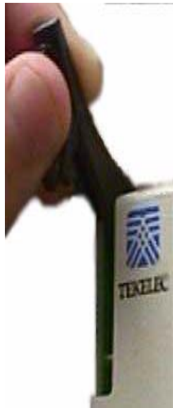
Figure 4-2. Push Inject/Eject Clamps Outward
