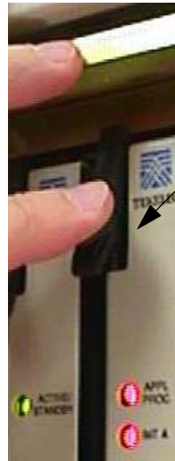
Figure 4-3. Push in Inject/Eject Clamps
