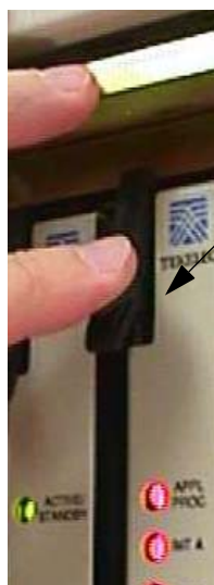
Figure 4-1. Push in Inject/Eject Clamps
