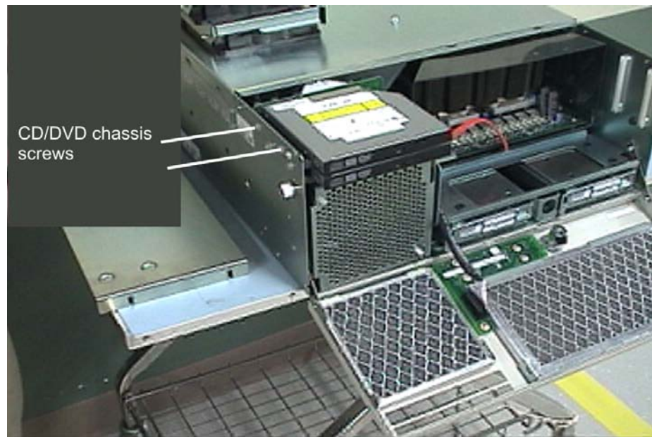
Figure 7-17. CD/DVD chassis screws
