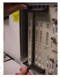
6. Pull the card directly towards you until it clears the card guides and guide rails.
