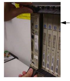
Push the card along the length of the card guides until the rear connector on the card begins engaging the mating connector on the backplane.
