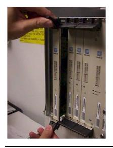
Push the card along the length of the card guides until the rear connector on the card begins engaging the mating connector on the backplane. 14. Press the faceplate of the card using constant pressure until you feel the card's progress cease.
