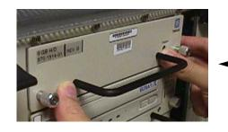
Press the faceplate near the areas where the handle is in \_ contact with the faceplate.
