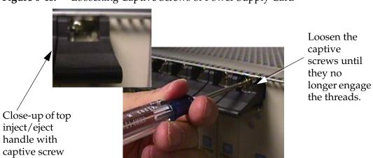
Figure 6-48. Loosening Captive Screws of Power Supply Card
