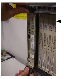
Push the card along the length of the card guides until the rear connector on the card begins engaging the mating connector on the backplane.
