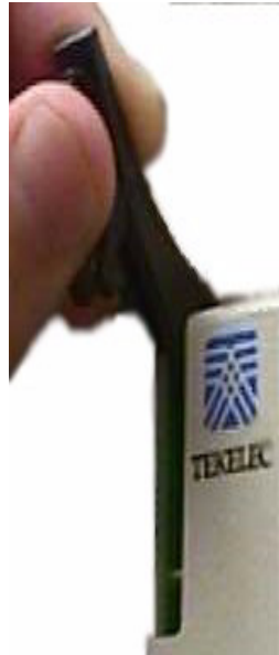
Figure 6-11. Push Inject/Eject Clamps Outward
