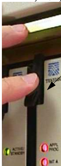
Figure 6-12. Push in Inject/Eject Clamps
