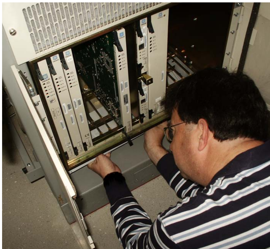
Figure 6-17. Insert fan tray bracket
