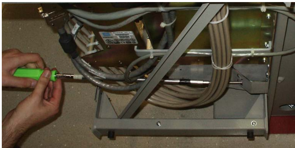
Figure 6-22. Tighten fan side bracket screws
