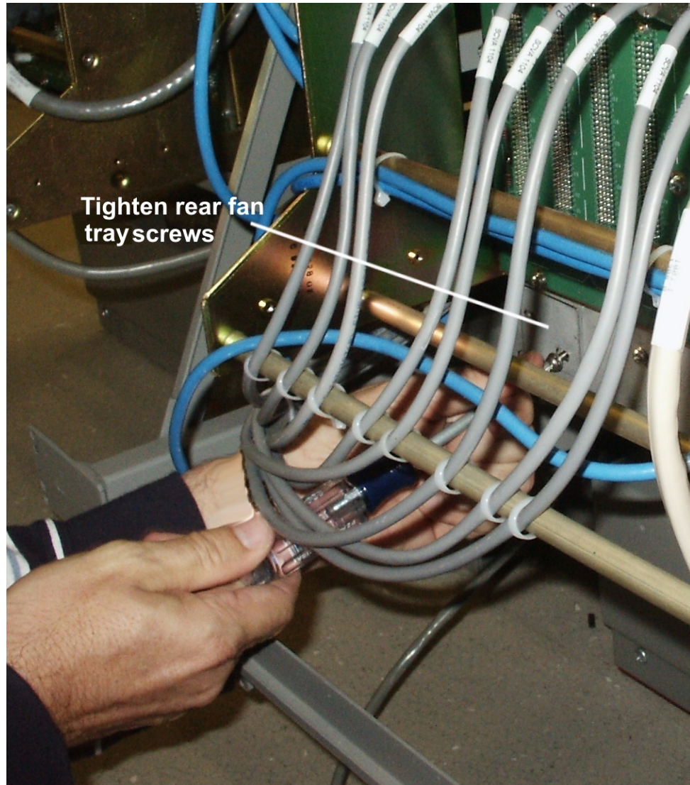
Figure 6-21. Tighten rear fan tray screws
