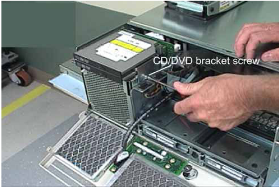
Figure 76: CD/DVD inside bracket screw location
