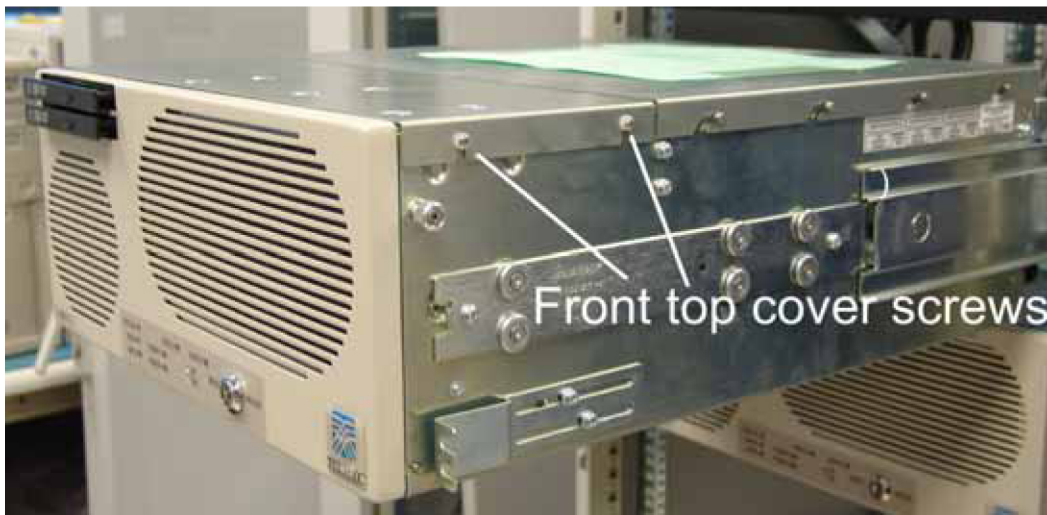
Figure 67: Front Top Cover Removal - Screw Locations
