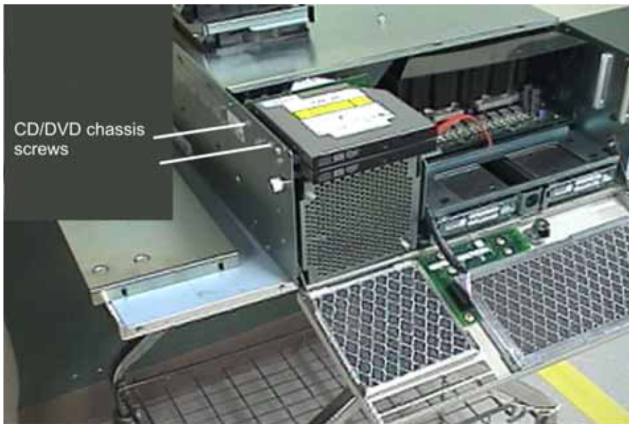
Figure 77: CD/DVD chassis screws
