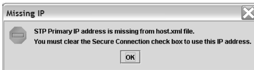
Figure 2-30. IP Address Warning Message
