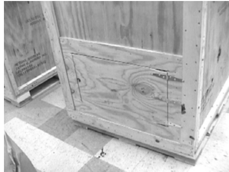
28.) Ensure that Rear access panel is closed and secured using the original 9/16" hardware.
