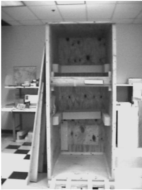
24) Replace brace and secure using the 9/16" hardware.
