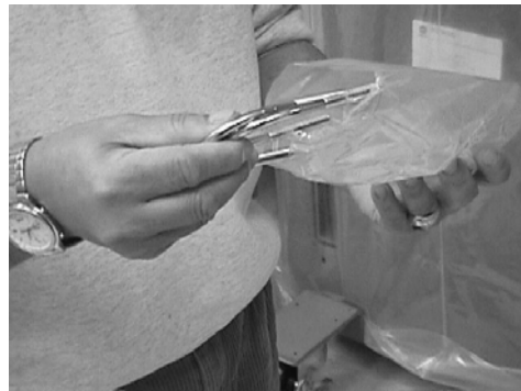
27) Place 2 "U" shaped keeper rings into a bag attached to the inside wall of the crate. If the Dolly Wheels stay with the system retain the 15/16 bolts and washers in the bag.
