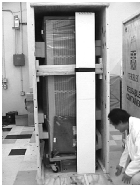
7.) Front Panel serves as the Loading / Unloading ramp. Position Ramp Text side up. Guide rails are on this top surface.
