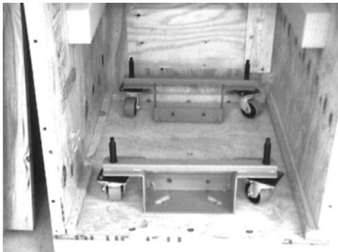
25) If Dolly wheels are no longer needed secure them to the base of the crate in the original positions using the 15/16" hardware.
